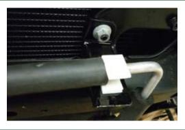
7. Place U-Bolts in position around chassis from inside out, in front of radiator.
