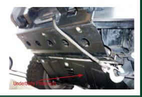
16. Attach right hand mud gaurd liner as shown and attach to washer bottle with cable tie.
