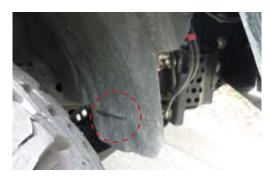
Attach left hand mud guard liner and secure with cable tie.
