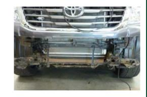
5. Remove bumper bar reinforcement.
