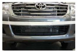
4 Cut along line and remove lower section of bumper.
