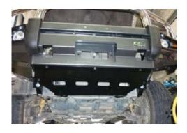
21. Trim left hand mudguard liner level with protection plate.
