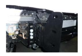
12. Place reinforcing brackets over U Bolts outside chassis and loosely fit M10 nuts, springs and flat washers.
