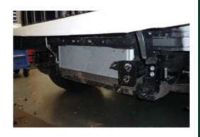
10. Place U-Bolts in position around chassis from inside out, in front of radiator.
