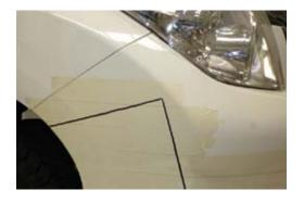
6. Mask a line across bumper level with the top edge of number plate recess and the bottom of the cut lines marked in previous step.
