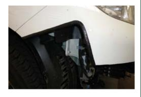
9. Remove aluminium bumper reinforcement and mounting brackets.
