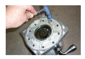
5. Re-install 10 bolts and tighten firmly. NOTE: Take care not to over-tighten.
