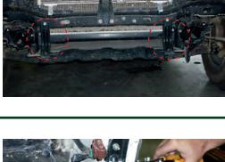
6. Using flare as a guide, mask another line towards the top of the bumper where flare piping contacts bumper bar, stopping 5mm short of the top edge.
