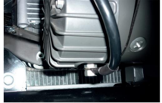
15. Run the positive and negative battery cables into the engine bay taking care to secure cables away from any sharp or moving objects. Connect negative battery cable to the main battery.
