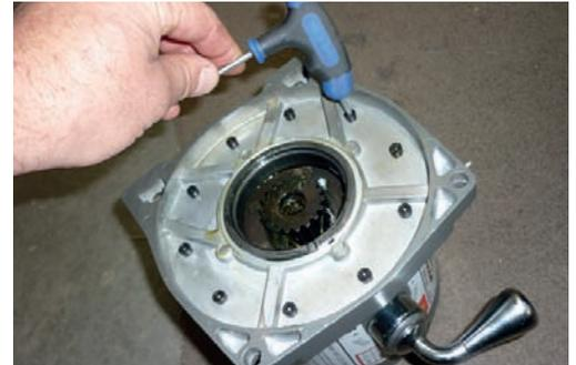
5. Re-install 10 bolts and tighten firmly.
