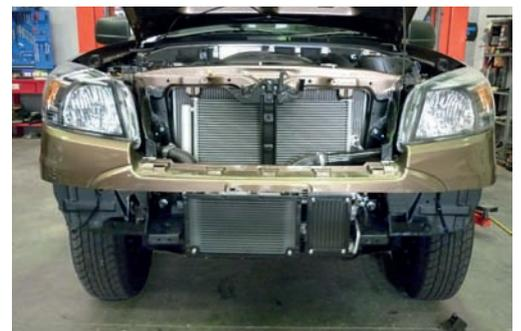
6. Place chassis bracket in position on chassis, making sure that bracket does not touch the vehicle body.
