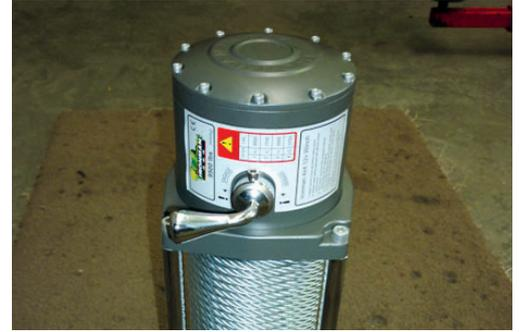
2. Undo and remove two chrome Allen head bolts which hold the gearbox to the tie rods.
