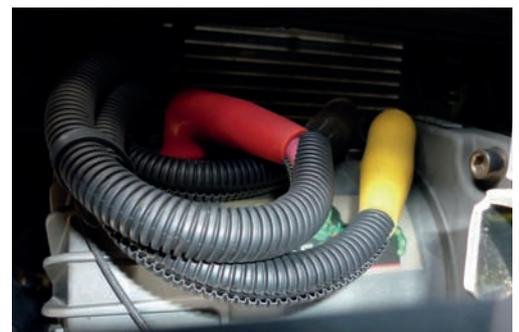
14. Connect the thin black earth wire and negative battery cable to the earth connection on the opposite side of winch motor.
