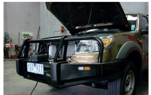
11. Align bull bar with vehicle and tighten all bolts. Allow approx. 20mm gap between bull bar wing and flare.
