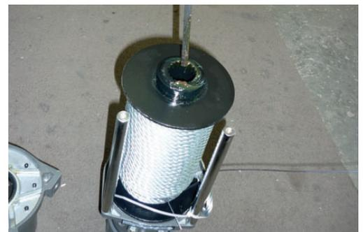
NOTE: Also make sure that the drum support bush remains in the end of the drum support housing with the locating tang in the correct position.
