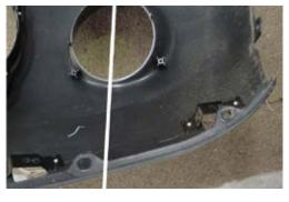
2. Cut to remove lower section of bumper bar.
