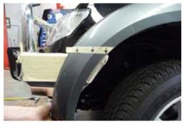
Fit protection plates underneath the bull bar using M8 bolts, spring washers and flat washers provided and trim guards liners to suit.
