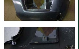
2. Cut to remove lower section of bumper bar.
