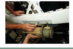
13. Connect three colour coded cables to the corresponding poles on winch motor.
