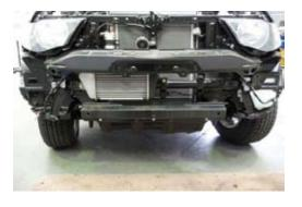
4 Remove front sections of mudguard liner and inner and outer support brackets.
