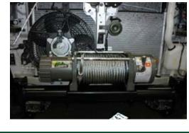
13. Connect three colour coded cables to the corresponding poles on winch motor.
