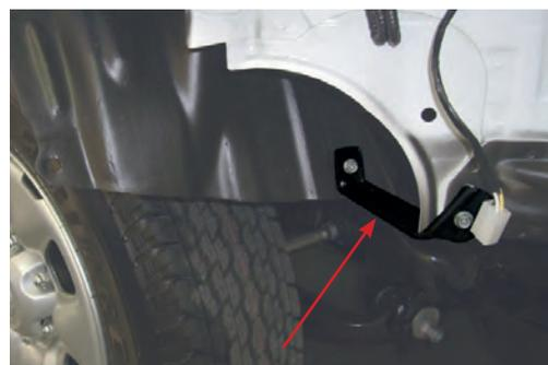
Note: Secure using a modified original lower bumper support bracket as shown.
