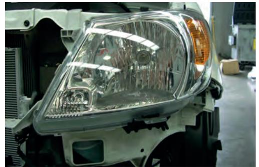
4. Remove plastic deflectors from between headlights and radiator opening.
