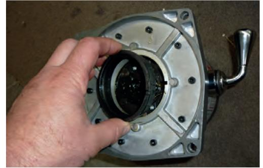
4. Undo and remove 10 Allen head bolts that hold the gearbox housing to the drum support housing and rotate the drum support housing to the desired location.
