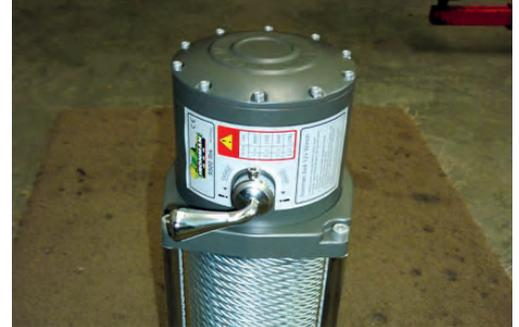
2. Undo and remove 2 chrome Allen head bolts which hold the gearbox to the tie rods.
