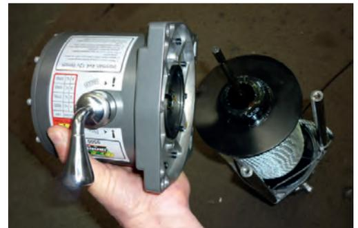
**NOTE:** If shaft comes out of cable drum remove it from the gearbox and place it back into the drum making sure it engages with the brake.
