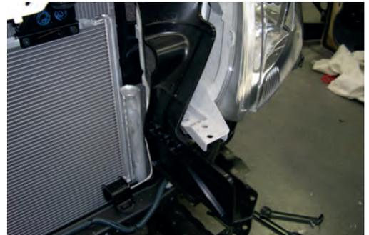
5. Remove plastic mud guard clips from lower mud guard lips.
