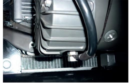
14. Run the positive and negative battery cables into the engine bay taking care to secure cables away from any sharp or moving objects.
