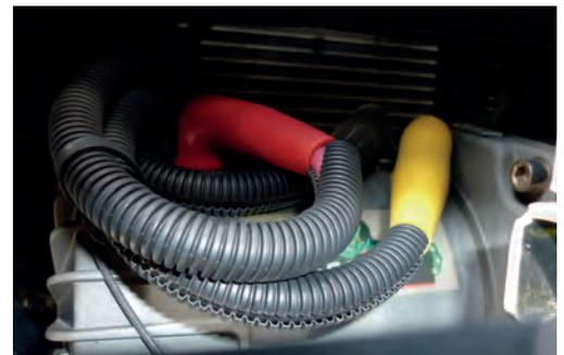
13. Connect the thin black earth wire and negative battery cable to the earth connection on the opposite side of winch motor.
