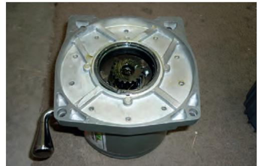
6. Refit gearbox to winch, refit and tighten Allen head bolts into tie rods.
