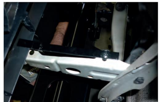
16. Fit protection plates underneath the bull bar using M8 bolts, spring washers and flat washers provided.
