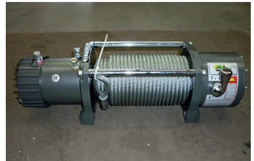
7. Bolt winch to cradle with gearbox to the left hand side of vehicle and cable spooling from bottom of the cable drum using bolts and washers provided.
