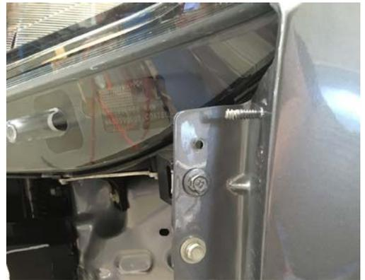
13. Unwrap bull bar. Check over riders and light assemblies are tight in bull bar before installation.
