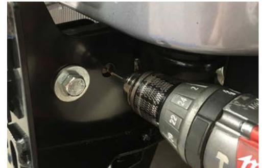
7. Install winch cradle as shown using hardware provided.
