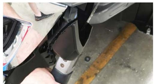
11. Remove bumper bar end brackets as shown.
