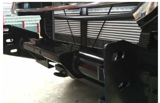
8. Remove bumper bar from grill. Mark cut lines on grill and remove lower section using air hacksaw or similar.
