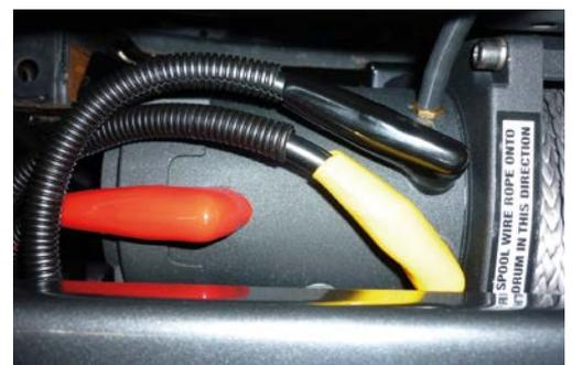
6. Connect the thin black earth wire and negative battery cable to the earth connection on the opposite side of winch motor.
