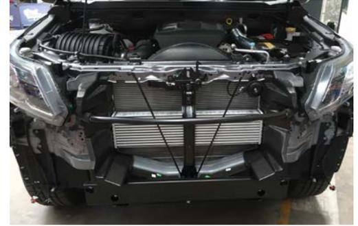
2. Remove grill, front bumper, bumper bar reinforcement, bumper bar support brackets and front protection plate from under chassis.
