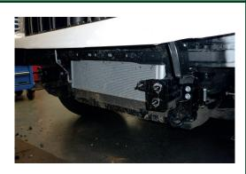
10. Hold mounting cradle in position and mark bumper in two positions as shown to allow clearance for brackets. Remove two sections 30mm high as shown.
