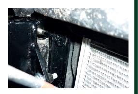
12. Attach mounting cradle to chassis using factory bolts and heavy duty flat washers.
