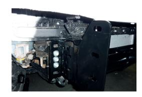
13. Place reinforcing brackets over U Bolts outside chassis and loosely fit M10 nuts, springs and flat washers.
