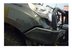
18. Once bull bar is aligned with vehicle and tightened, drill through pinning holes (circled in red) between bull bar and chassis bracket and secure with bolts, washers and nuts provided.
