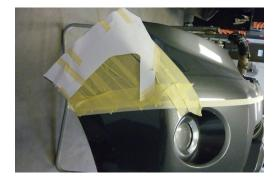
6. Mask a line across bumper level with the top of fog light opening, top of number plate mount and the bottom of lines marked with template in previous steps.
