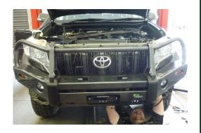
17. Align bull bar with vehicle and tighten all bolts.
