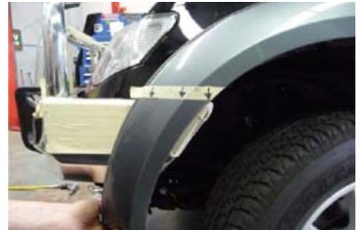
14. Remove flares and cut along line previously marked.
