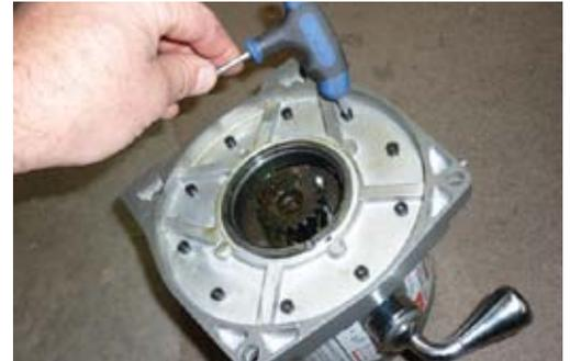
5. Re-install 10 bolts and tighten firmly.
