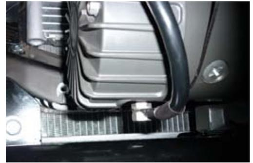
15. Run the positive and negative battery cables into the engine bay taking care to secure cables away from any sharp or moving objects.
