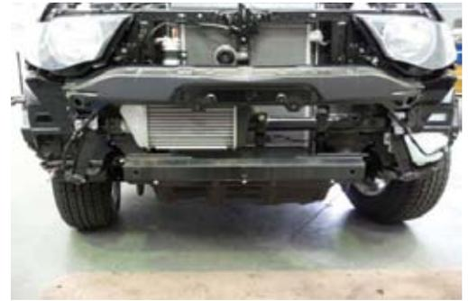
4. Remove front sections of mudguard liner and inner and outer support brackets.
