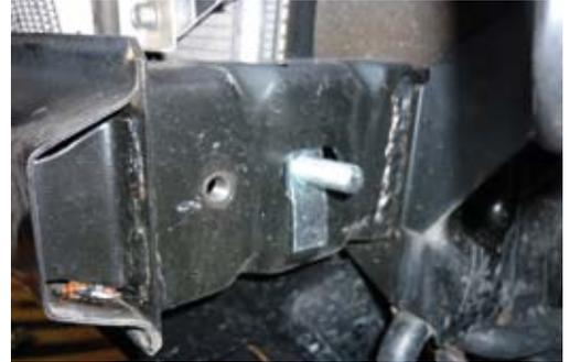
6. Attach chassis strengthening brackets as shown using nuts, bolts and U-bolts provided.
