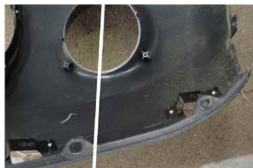
2. Cut to remove lower section of bumper bar.
