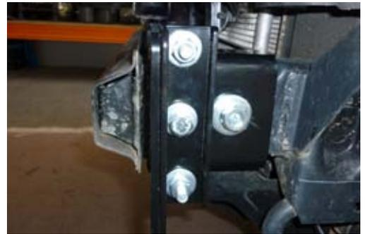
7. Install mounting cradle as shown. Tighten all bolts.
