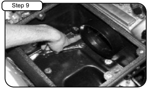
Step 9 Place housing into vehicle and tighten using 12mm socket or wrench. With M8 nut and washer provided tighten down housing onto isolation mount with 13mm wrench.
