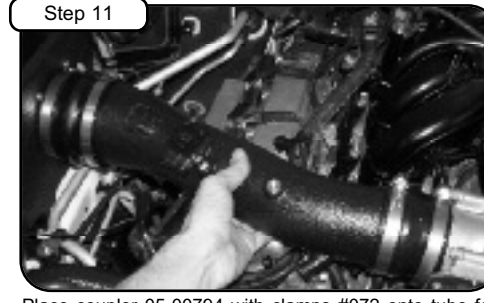
Step 11 Place coupler 05-00794 with clamps #072 onto tube for adaptor side of housing. Then place coupler 05-00815 with clamps #052 and #048 onto tube for throttle body side. Install loose to allow repositioning.
